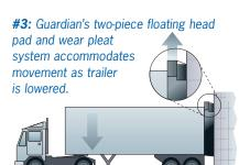
Guardian is the ideal solution for air-ride suspension trailers, which can move up and down as much as 8" during loading/unloading.
